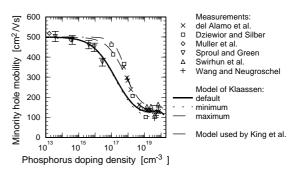
Fig. 2: Minority hole mobility as a function of phosphorus dopant density. The model of Klaassen [15] is modified to fit the smallest and largest measured values.
