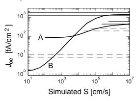
Fig. 3: Simulated  $J_{oe}$  of the highest (A) and lowliest (B) doped emitter of Cuevas et al. The error bounds of the measured  $J_{oe}$  of metal coated and oxide passivated surfaces are given by the solid and dashed lines, respectively.
