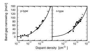
Fig. 1: Measured [15] (symbols) and calculated [6] (line) band gap narrowing as a function of phosphorus dopant density.
