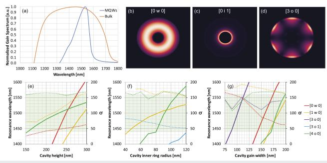
FIG. 2. (a) Normalized gain spectrum of bulk and MQW gain medium, the transverse intensity profiles of three supported modes (b) [0 w 0], (c) [0 i 1], and (d) [3 o 0], and modal resonance wavelength (solid line) and Q-factor (dashed line) shift over (e) cavity height, (f) cavity inner ring radius, and (g) cavity gain width.
