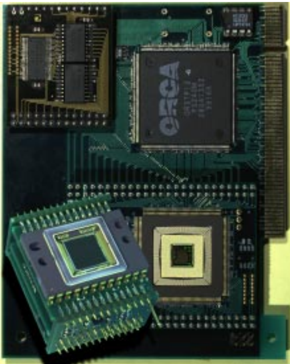
Miniaturized head of the 1-Megapixel CCD video camera. In the background: PCI card containing the image signal processor ASIC (open package), an FPGA with PCI interface, and SD RAMs for intermediate storage.
